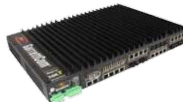
**10KT Managed Switches** include industry-leading IEEE 1588 v2 precision timing for utility applications, the first dual hot-swappable power supplies in a 1U rack-mount switch, 61850-3 compliance, and up to 36 ports in 10 slots, highly configurable to meet the needs of each installation.
