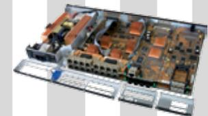
Conformal coating refers to a protective coating designed to conform to the surface of an assembled printed circuit or PWA. This coating protects the circuitry from humidity, moisture, dust, and corrosion which can be caused by exposure to extreme environments. Both 5-mil and 14-mil silicone are available.
